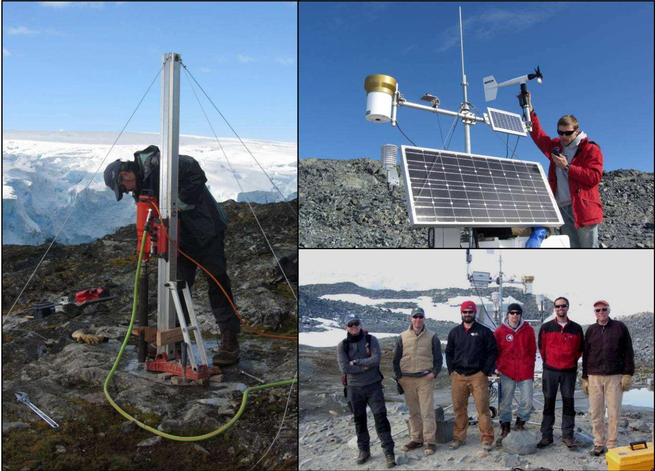
**The Bockheim group (G-239) drilled their 15-meter bore hole at the top of Amsler Island during their time at Palmer Station this month. Temperature sensors placed in the bore hole will reveal the depth of the active (permafrost) layer in the Palmer area. The group also serviced the weather station they installed last season and mapped surficial geology, soil, and vegetation on the island.** *Image Credit: Janice O'Reilly*
